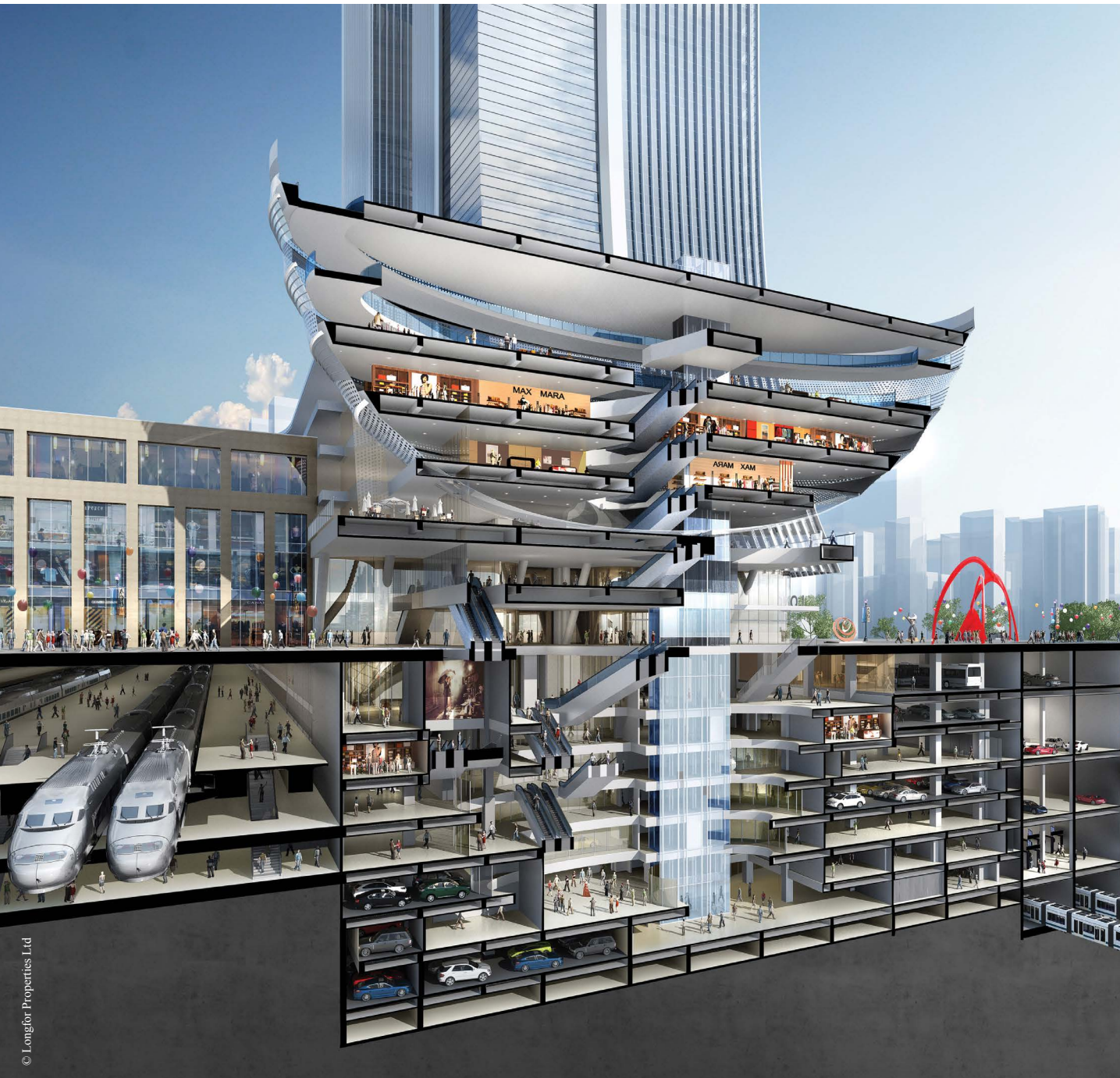
The centrally located lift/elevator system serves all floors of the underground and aboveground parts of the building.
